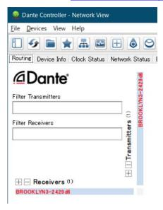
When the Dante module could not be booted in the failsafe mode, it is shown as a fixed Device Name like "Y001-Yamaha-DM3-xxxxxxx" with red text in the network grid view of Dante Controller. In this case, follow the procedure "Recovery of the Dante module (without the failsafe mode)" (page 8) to recover the system.
