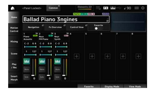
When the Panel Lock function is engaged, all operations will be unavailable, except the keyboard, pedals, Master Volume, Super Knob, Pitch bend wheel, Modulation wheel, Ribbon controller, and, of course, disengaging the unlock operation. This lock also applies to touchscreen operations.
