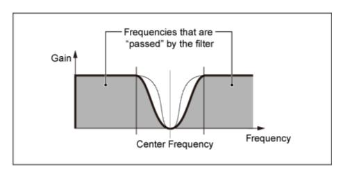
BEF12: -12 dB/oct Band-Eliminate Filter.
