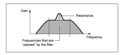
**BPFw**: A −12 dB/oct BPF that combines HPF and LPF filters to allow wider bandwidth settings.
