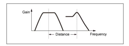
Lower Cutoff Frequency is set directly on the display (and Higher Cutoff Frequency is automatically set)
