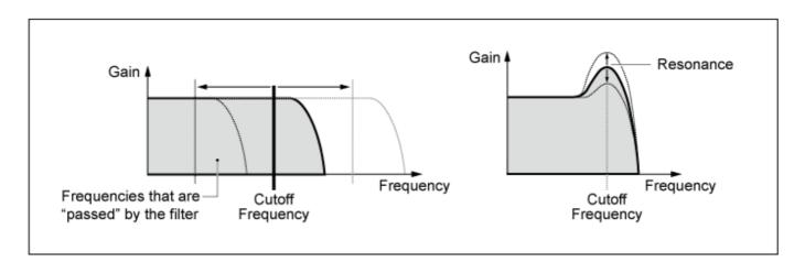
**LPF24D**: A dynamic –24 dB/oct Low-Pass Filter with a characteristic digital sound. Compared to the LPF24A type, this filter can produce a more pronounced Resonance effect.
