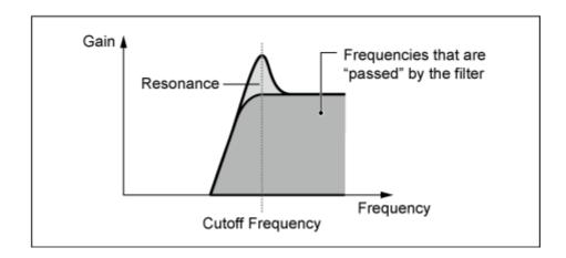
HPF24: -24 dB/oct HPF18: -18 dB/oct HPF12: -12 dB/oct HPF6: -6 dB/oct
