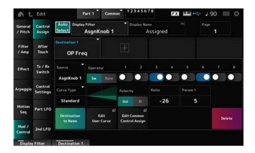
The screen here is basically the same as the one opened from  $Mod/Control \rightarrow Control Assign$  on the Part Edit (AWM2), except that the available Destination settings are different. For a list of settings, refer to the Data List.
