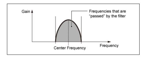
**BPF12D**: The combination of a -12 dB/oct HPF and LPF with a characteristic digital sound.
