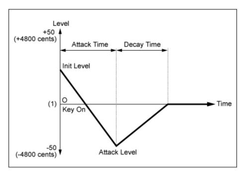
(1) Pitch (frequency) set to Coarse Tune and Fine Tune
