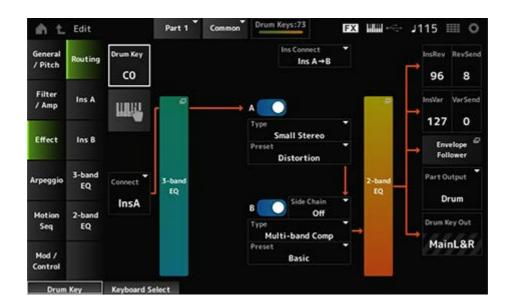
Basically, this is the same screen as  $Effect \rightarrow Routing$  in  $Part\ Edit\ (AWM2.)$  The parameters added to  $Drum\ Part\ Edit\ (AWM2)$  are shown below.
