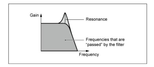
**LPF24A**: A digital dynamic Low-Pass Filter with characteristics similar to a 4-pole analog synthesizer filter.
