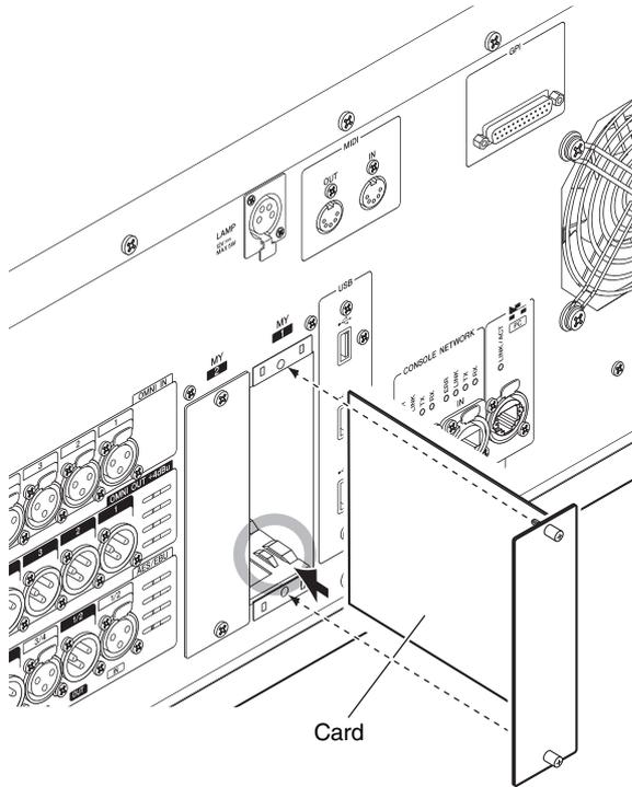
4. Fasten the card using the screws attached to the card.
