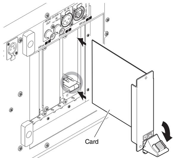
Push the card all the way into the slot so that the connector at the end of the card is correctly inserted into the connector inside the slot.
