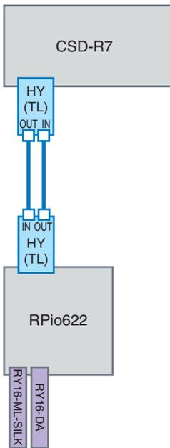
Use fiber optic cables to connect the TWINLANe IN/OUT connectors on the HY card installed on the digital mixing console to the TWINLANe IN/OUT connectors on the HY card installed on the I/O rack.
