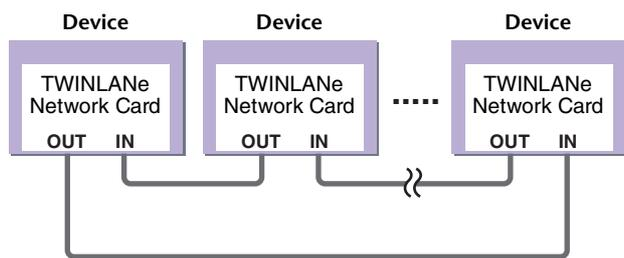
A TWINLANE network uses a ring topology, which provides redundancy in case of broken cables. If a cable in the network breaks down for some reason, the signal will be automatically re-routed and audio will flow without interruption. Even if a device in the network malfunctions, other working devices will be able to continue communicating.
