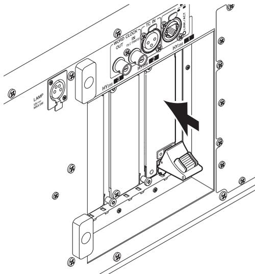
**4. Pull up the card installation lever to lock in the card.**
