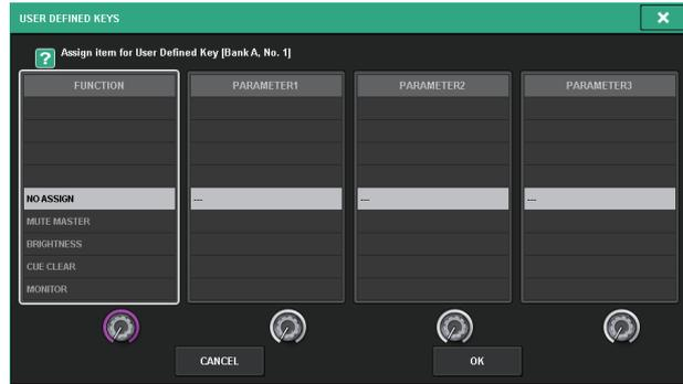
The highlighted item in the middle of the list is the item that is selected for operation. Press the screen encoders located below the list to scroll the list upward or downward.
