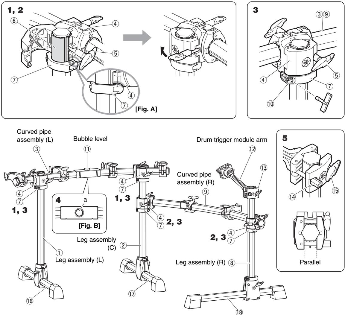
1. Attach the curved pipe assembly (L) ③ to the leg assemblies (L) ① and (C) ② and secure. Loosen the fixing bolts ⑤ on the open clamps ④ attached to both ends of the curved pipe assembly (L) ③, then align the sleeve ⑥ and memory clamp ⑦ on the leg assemblies and attach. When attaching, make sure that the nub on the memory clamp ⑦ is aligned with the indent on the open clamp ④ (Fig. A).
