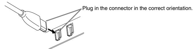
**NOTE** For optimum results, use an IEEE1394 cable shorter than 4.5 meters.
