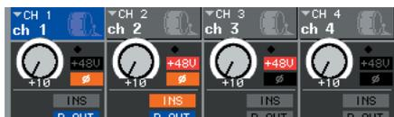
**4** While performing on the mic or instrument, use the Centralogic section’s multifunction encoders 1–8 to adjust the HA gain of each channel.
