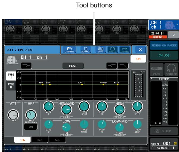
There are three types of popup window, “1 ch” windows that show only a specific channel, “8 ch” windows that show the currently selected group of eight channels, and “ALL” windows that show all channels in a single view. You can switch between these using tabs.
