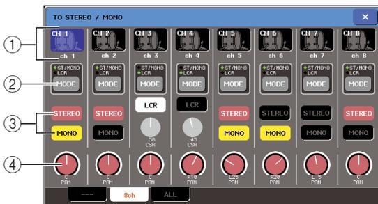
Here you can control the on/off and pan/balance settings of the signal sent from input channels to the STEREO (L/R) bus and MONO (C) bus, in groups of eight channels.
