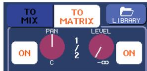
For an INPUT channel, the right knob will adjust the common send level to the two MATRIX buses, and the left knob will adjust the panning between the two MATRIX buses. Turning the left TO MATRIX SEND LEVEL knob toward the left will increase the amount of signal sent to the odd-numbered MATRIX bus, and turning it toward the right will increase the amount sent to the even-numbered MATRIX bus.
