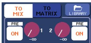
If necessary, you can specify two adjacent odd-numbered/even-numbered MIX buses as a stereo bus and link the main parameters (→ p. 234).
