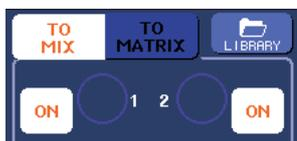
If the send-destination MIX bus is a VARI type, the TO MIX SEND LEVEL knob is displayed in the same color as the corresponding encoder of the SELECTED CHANNEL section. In this case, you can use the corresponding encoder of the SELECTED CHANNEL section to adjust the send level.
