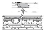
3 Insert the six new batteries, being careful to follow the polarity markings on the inside of the compartment.
